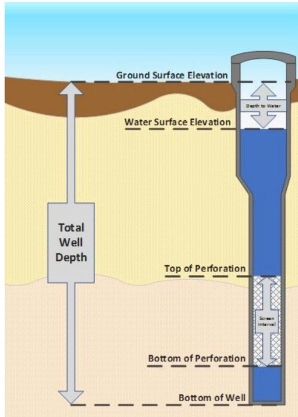
**Figure 7-1. Diagram of Key Groundwater Monitoring Well Measurements**
