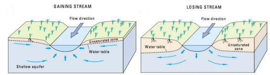
Figure 5-90. Gaining and Losing Surface Water Features
