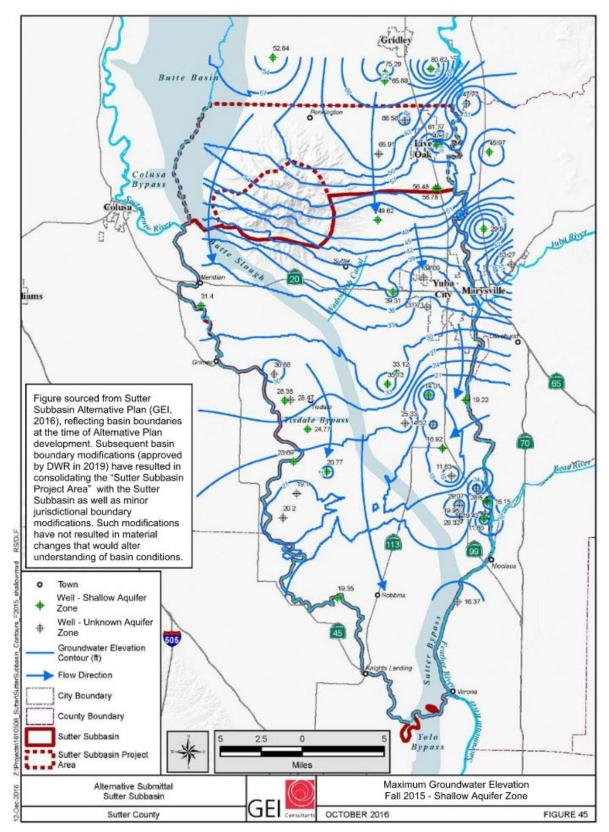
Figure 5-77. Groundwater Elevation in Shallow Aquifer Zone, Fall 2015
