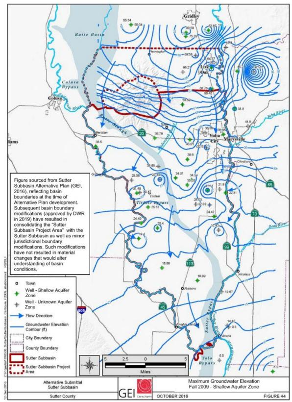
Figure 5-54. Groundwater Elevation in Shallow Aquifer Zone, Fall 2009
