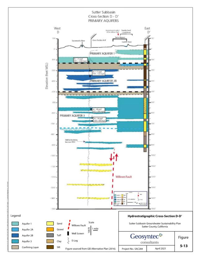
Figure 5-13. Hydrostratigraphic Cross-Section D-D'
