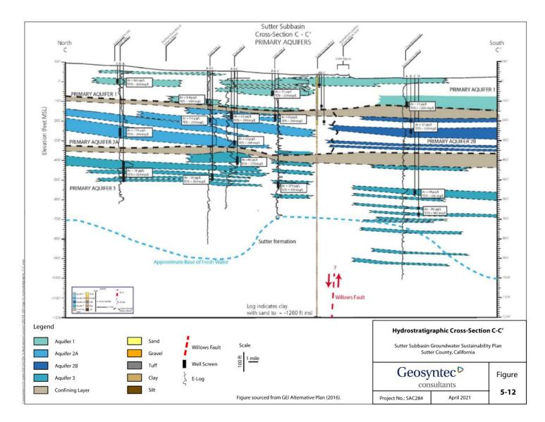
Figure 5-12. Hydrostratigraphic Cross-Section C-C'
