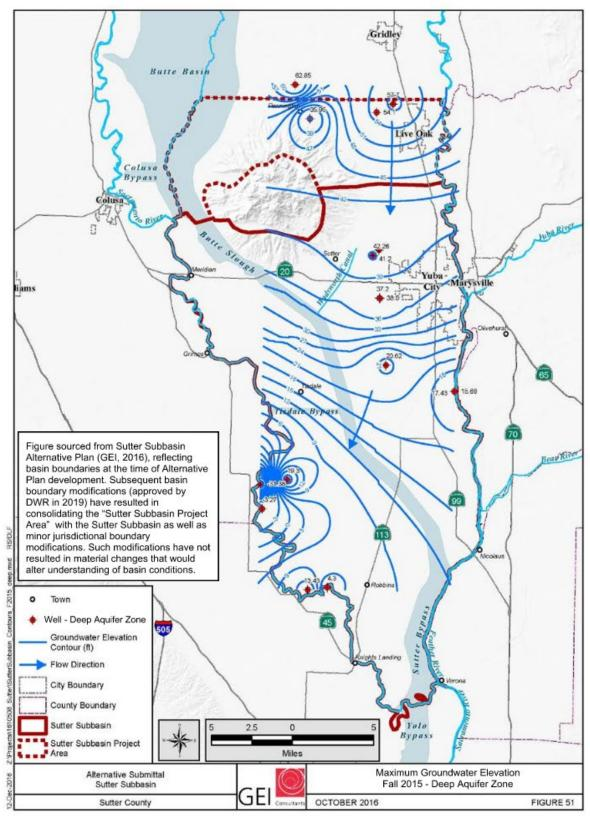
Figure 5-79. Groundwater Elevation in Deep Aquifer Zone, Fall 2015
