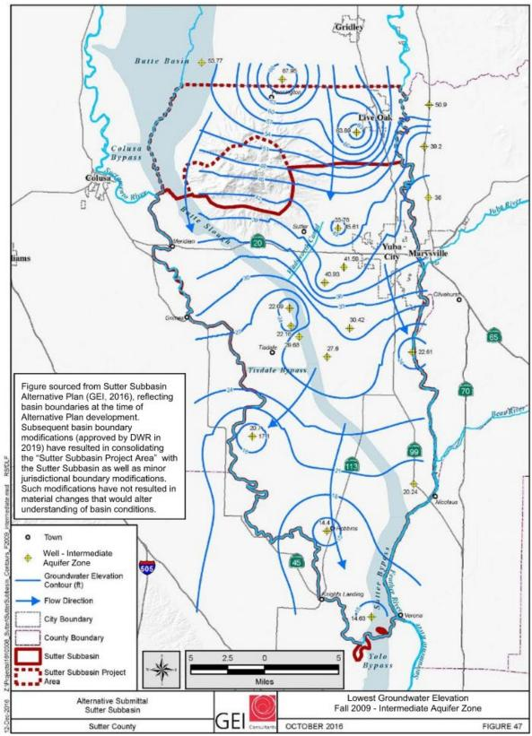
Figure 5-55. Groundwater Elevation in Intermediate Aquifer Zone, Fall 2009
