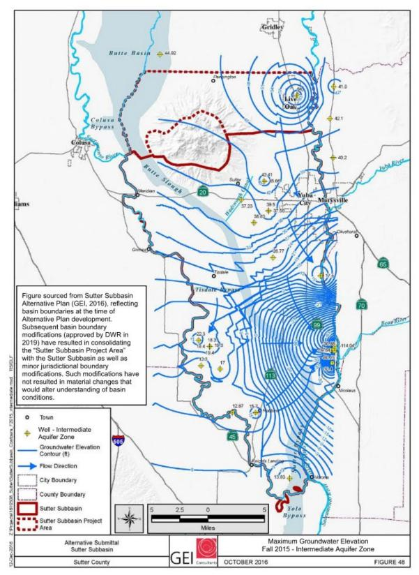
Figure 5-78. Groundwater Elevation in Intermediate Aquifer Zone, Fall 2015
