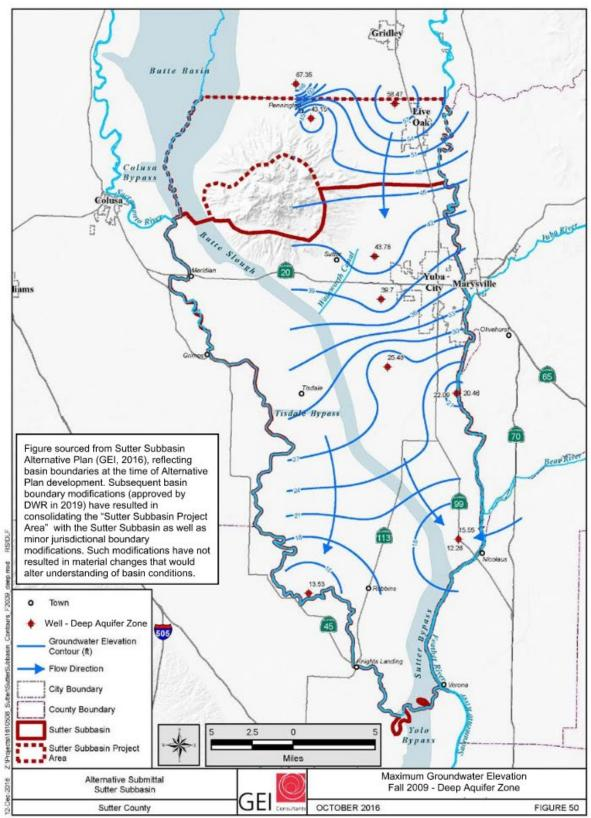
Figure 5-56. Groundwater Elevation in Deep Aquifer Zone, Fall 2009
