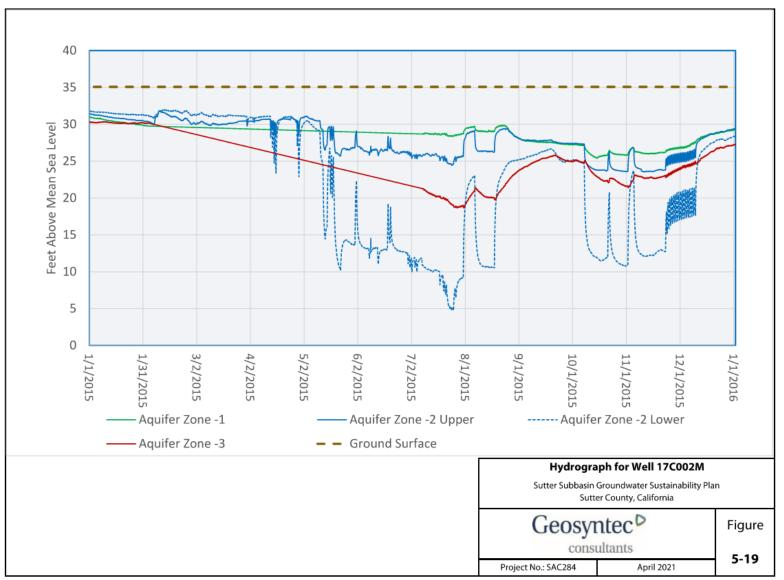
Figure 5-19. Hydrograph for Well 17C002M
