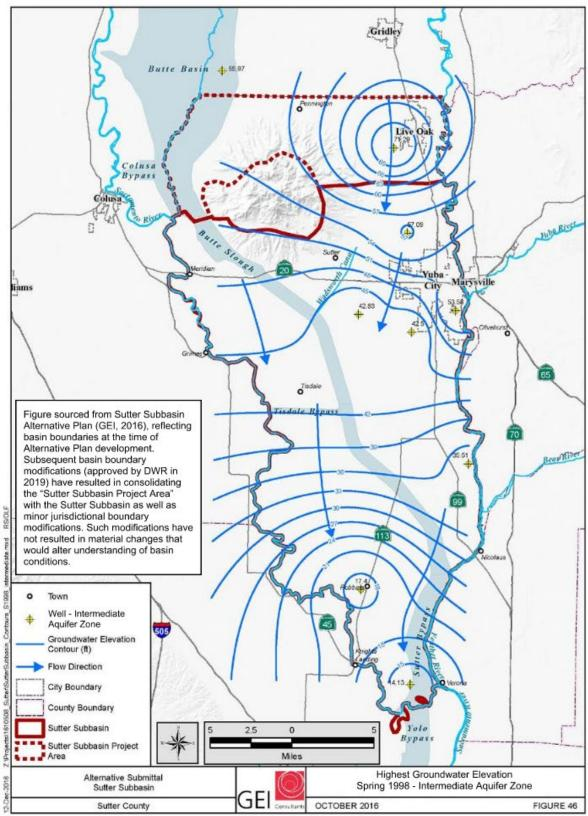
Figure 5-52. Groundwater Elevation in Intermediate Aquifer Zone, Spring 1998
