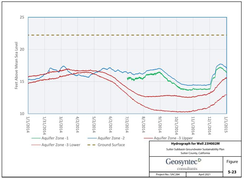
Figure 5-23. Hydrograph for Well 23H002M
